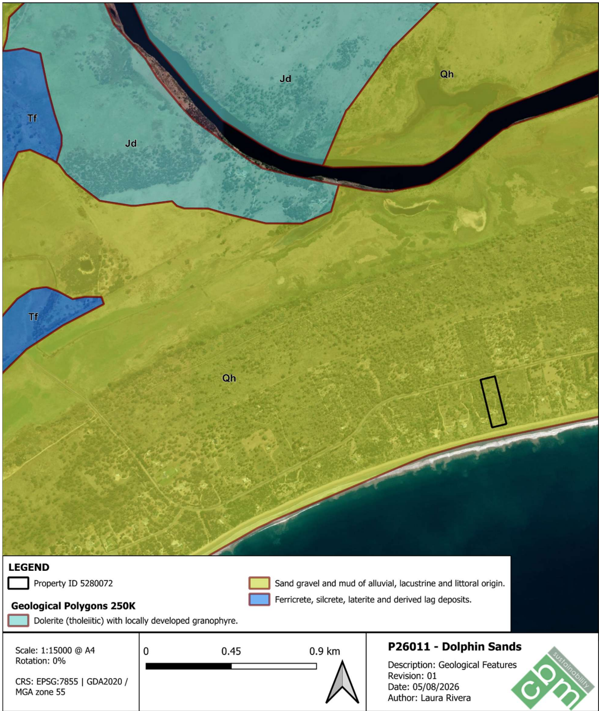
Figure 2. Geology features for the site and surrounding
